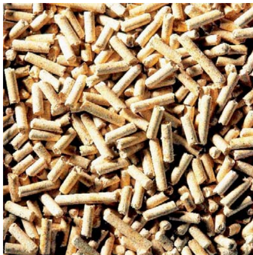
Fig. 7 Ligning is responsible to keep the sawdust tight
