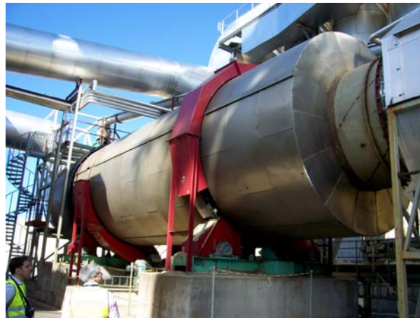
Fig. 2 drum drier installed at a pellet mill
