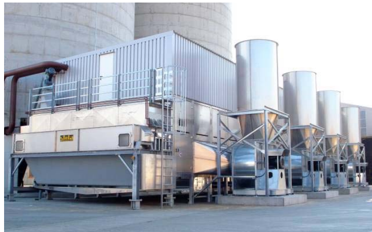
Fig. 3 low-temperature belt drier for sawdust
